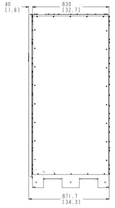
Figure 3-2. UPS Cabinet Dimensions (Right Side View)
